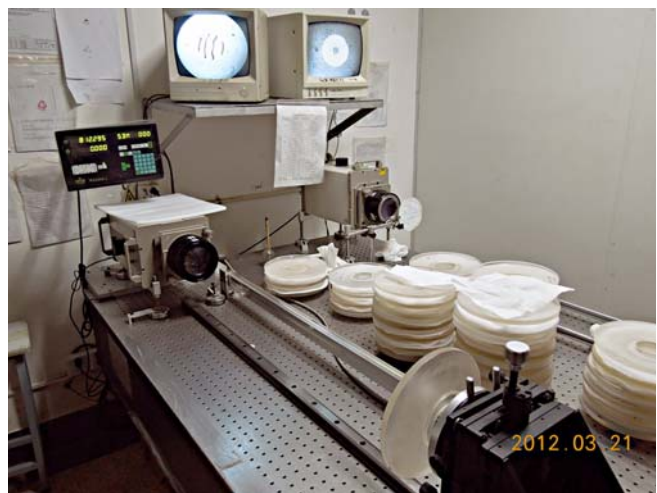
Figure 10. We test all of our primary mirrors on an optical bench by means of laser interferometry. In the picture, stacks of polished primary mirrors await testing on one of our optical test benches.
