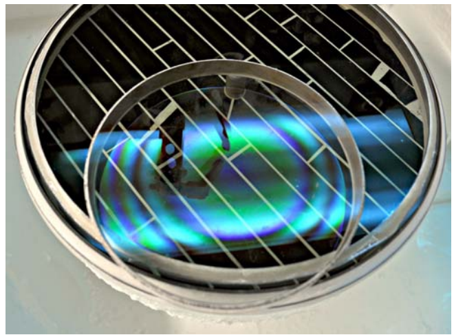
Figure 7. Matchplates use interference fringes to check the radius and smoothness of the correction. In this picture, you see a corrector blank attached to a master block. The matchplate rests on top; interference fringes appear as green and blue circles. The circular pattern indicates a difference in radius.
