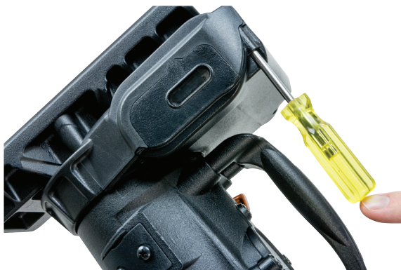
Figure 12 Removing the gear cover
